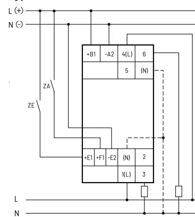
When the (N) is connected, the contact switching is active in the zero crossing.
